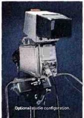
But whether you're indoors or out, the AK-750B performs superbly with a S/N ratio of 50dB, and horizontal resolution is 500 lines at center (recommended illumination of 200 footcandles at f/4). There's even a + 6dB gain for minimum illumination of just 15 footcandles at f/1.8.
